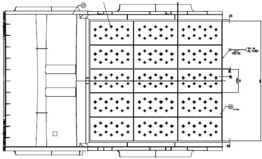
Each Wear plate – Floor (exploded view) as shown below to be welded as per procedure in base floor of dump body.
