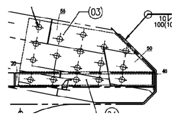
Details of Wear plate –Side, Qty- 02nos. Each wear plate-side to be welded as per procedure in LH& RH sides of Dump body.
