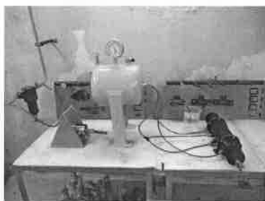
FA-2: Sealing test set up
