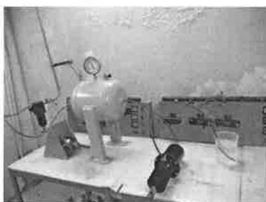
FA-1 Cylinder: Sealing test set up
