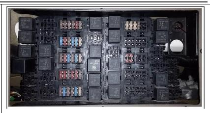
Suitable rating of fuses (i.e., 5Amps, 8Amps, 16Amps, 25Amps Etc) and relay to be used for protection against short circuit and over load protection of electrical and electronics component of dash board control and electrical system of the equipment.
