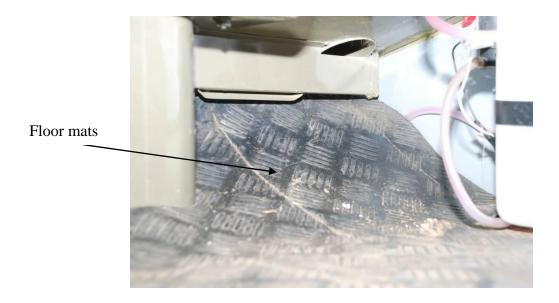
The floor mats are of 3 piece construction to be provided with 10 mm thick insulation. Rexin to be used with paste to fix the floor mat on the tunnel surface. The insulation shall be such that the cabin complies with NVH levels as per CMVR norms.
