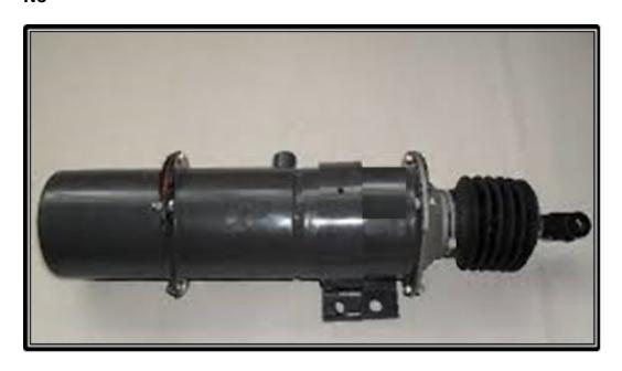
4) P/N: 131612193004 - BRAKE CYLINDER (REAR AXLES-I & II) - Qty/Ept = 4 No
