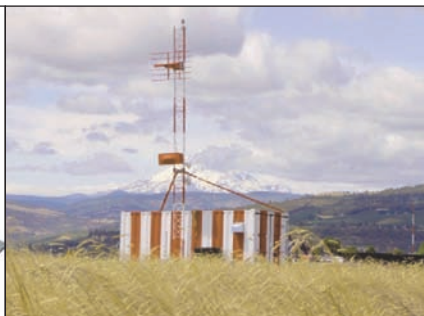
Transponder Landing System (TLS) ground base precision system.
