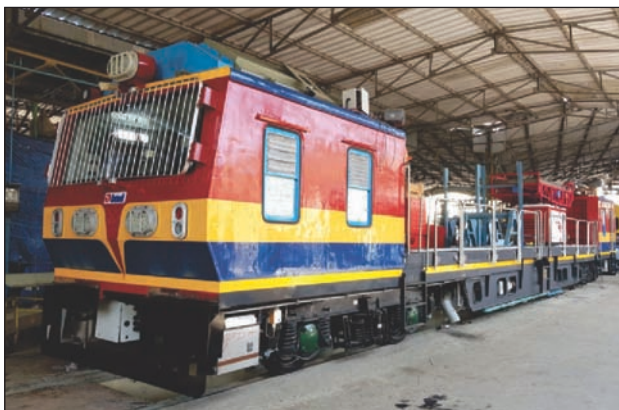
First time in India BEML has indigenously designed & developed Catenary Maintenance Vehicle for Rail routes of Metro
